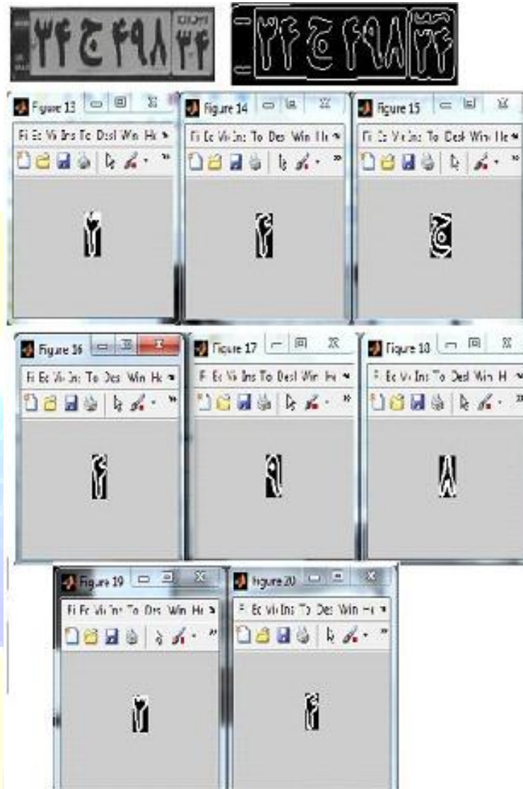
Figure 7: phases of Letters separation algorithm
