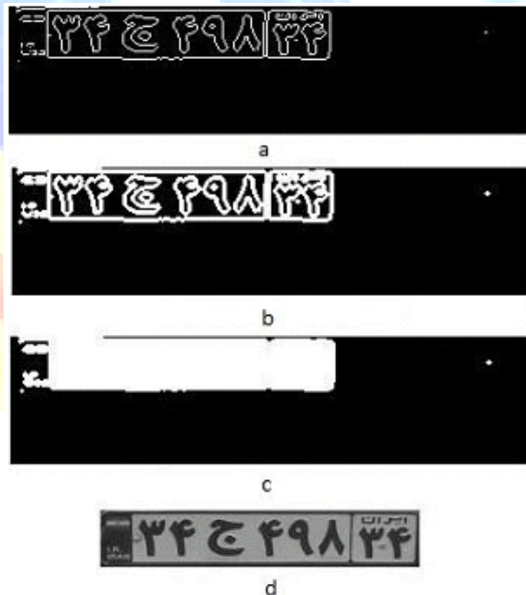
Figure 6: license plate separate stages from image (a: The edge detection of an image, b: edge strengthens, c: filling holes caused, d: license plate extraction from image)
